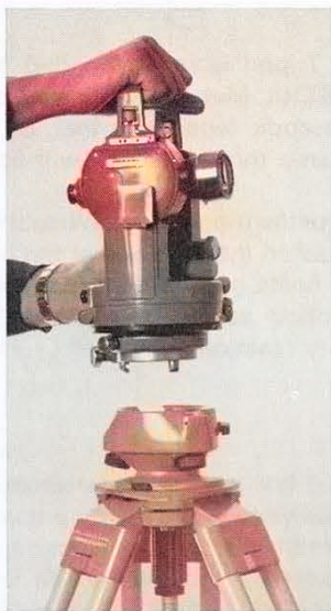
Fig. 5 Placing the T1 in the GST70 Centring Tripod
