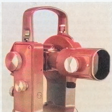
Fig. 11 Parallel Plate Micrometer GPM5. The counterweight balances the telescope
